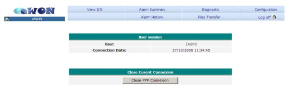
You can use the *Close PPP Connection* button to close the remote connection. Bear in mind that the connection will be interrupted after the *Idle time before hanging up*, will be elapsed (in case of inactivity).
