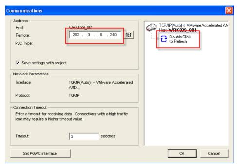
Enter the IP address of your eWON (Ethernet, PPP or Internet address), and double-click the *Refresh* option to see your PLC device. Following our example, we can now use both 202.0.0.240 or the local IP address of your eWON.
