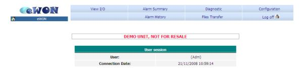
The menu bar on the top of the *Main* page allows you to navigate through the different displays and configuration pages of your eWON.
