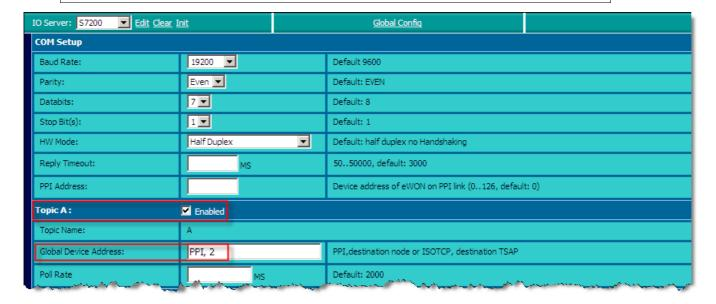
Select IO Server **\$7200**, enable **Topic A** and insert the **Global Device Address**. (PPI,2=the Tag will be polled at address 2 through the PPI connection).
