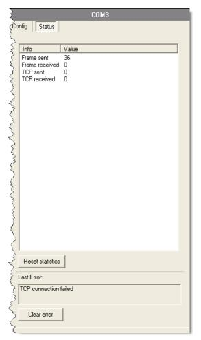
The **Status** area can be used to monitor the status of the eVCOM connection:
