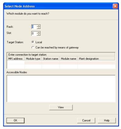
Click on the View button to display the MPI master nodes of the network.
