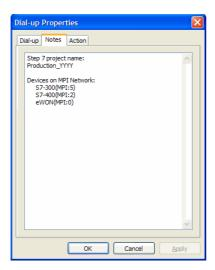
This window will allow you to encode some information that will be useful for the remote connection. For example, the name of the involved Step7® project or the addresses of the PLC which can be reached through the remote connection, ...
