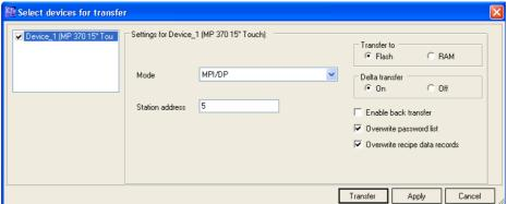
In the Transfer window set the **Mode** to MPI/DP, and enter the **Station address** of your device (5, in our example).
