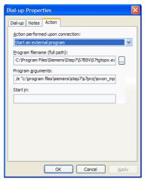
This window will allow you to configure the action that will be performed once the remote connection is established.
