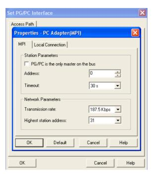
In the  $\emph{MPI}$  section, set the **Transmission rate** to 187.5 Kbps and click on the  $\emph{OK}$ button.
