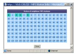
This table will show you the different MPI/Profibus Master devices detected by the MPI chip of the eWON. The detected MPI/Profibus devices are represented with a green square.
