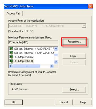
In the *Access Path* section, select the *PC Adapter (MPI)* and click on the *Properties* button.
