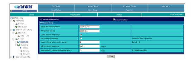
Check the **Server enabled** box for the PPP Incoming Connection.
