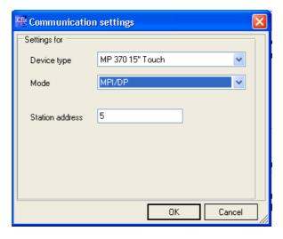
For the communication **Mode** select MPI/DP, and enter the Station address of your Siemens Panel (5, in our example). Click on **OK**.
