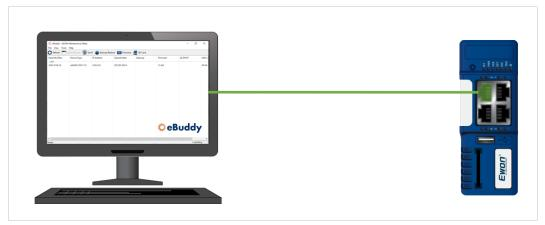
Fig. 27 Connect the computer directly to the Ewon
