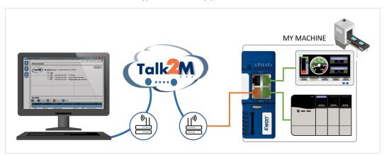
Fig. 11 Serial and Ethernet links between Ewon and Omron
