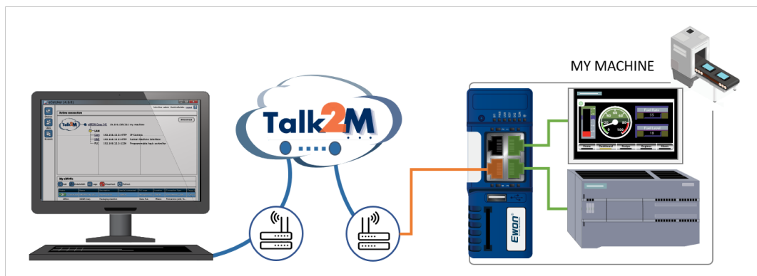
Fig. 11 MPI/Profibus and Ethernet ISOTCP link
