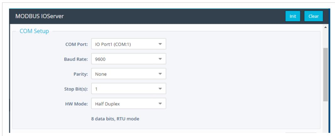
The screenshot shows the 'MODBUS IO Server' configuration interface. At the top right, there are 'Init' and 'Clear' buttons. The main section is titled 'COM Setup' and contains five dropdown menus for configuration: 'COM Port' (set to 'IO Port1 (COM:1)'), 'Baud Rate' (set to '9600'), 'Parity' (set to 'None'), 'Stop Bit(s)' (set to '1'), and 'HW Mode' (set to 'Half Duplex'). Below these settings, it indicates '8 data bits, RTU mode'.
