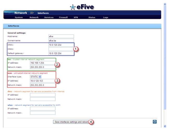
In the LAN section, replace the default address and Network mask by the one you want to use.
