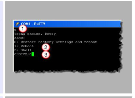
5. To **reset the unit to its factory settings** (IP 10.0.0.153 and the admin password to admin) type 0 and hit [enter]. Wait for the reboot to complete (takes some time).
