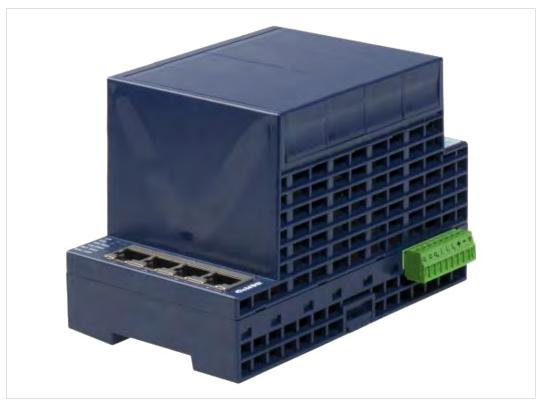
Fig. 1 Housing of the Flexy 201 Base Unit with its Original 4 Slot Fillers
