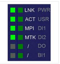
Fig. 14 LED Panel of the Flexy 103 & 203
