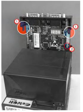
Fig. 17 Slot Removal
