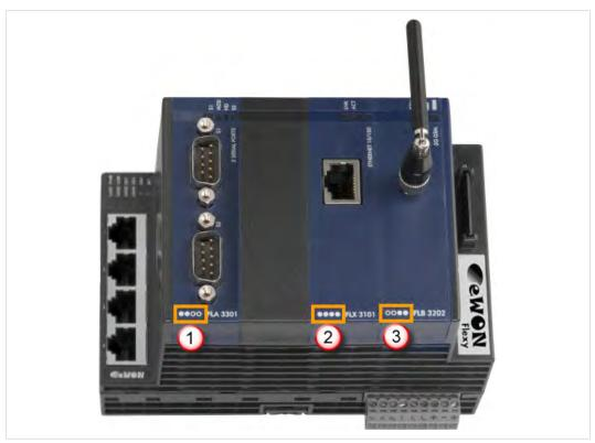
Fig. 16 Slot Compatibility Markings
