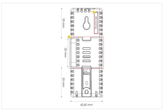
Fig. 1 DIN rail mounting position
