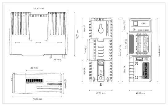
Fig. 5 Mechanical dimensions of the Ewon Cosy 131
