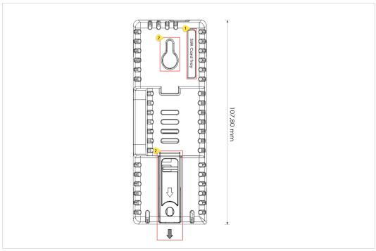
Fig. 2 Wall mounting position
