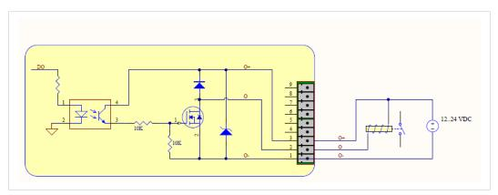
Fig. 14 External wiring for the Digital Output
