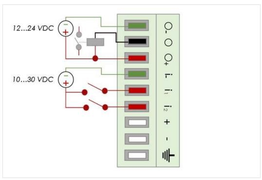
Fig. 13 Current scheme of the main connector
