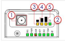
Fig. 9 Status LEDs representation – Wi-Fi model
