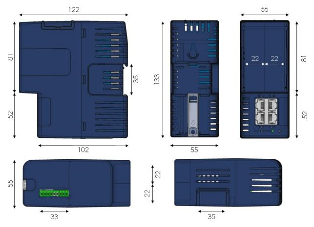
Figure 2. Mechanical Dimensions
