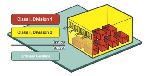
The standard Ewon® Flexy 205, can only be placed and used in the green area: OrdLoc.
