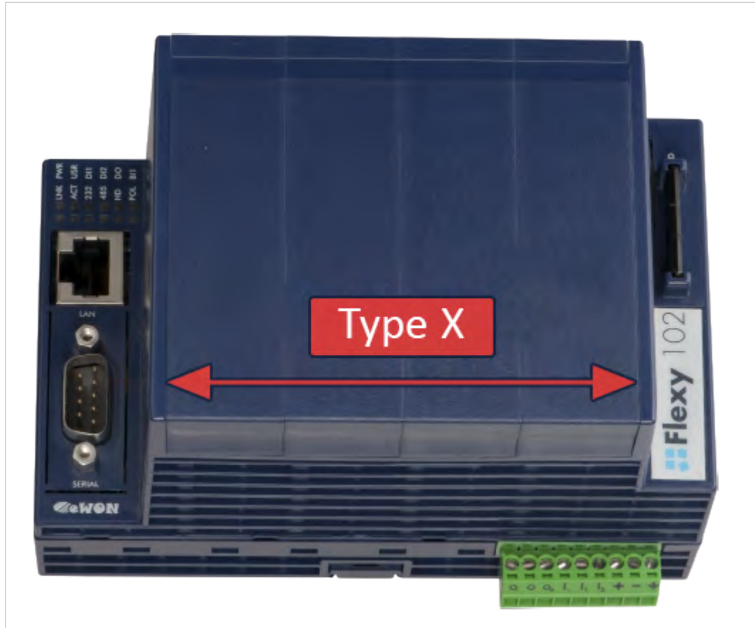
Fig. 8 Position of the "Type X" Slots on a Flexy 10x & 20x.
