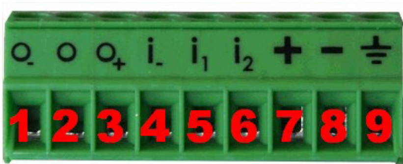
Figure A.1. The Ewon® Cosy+ Female connector
