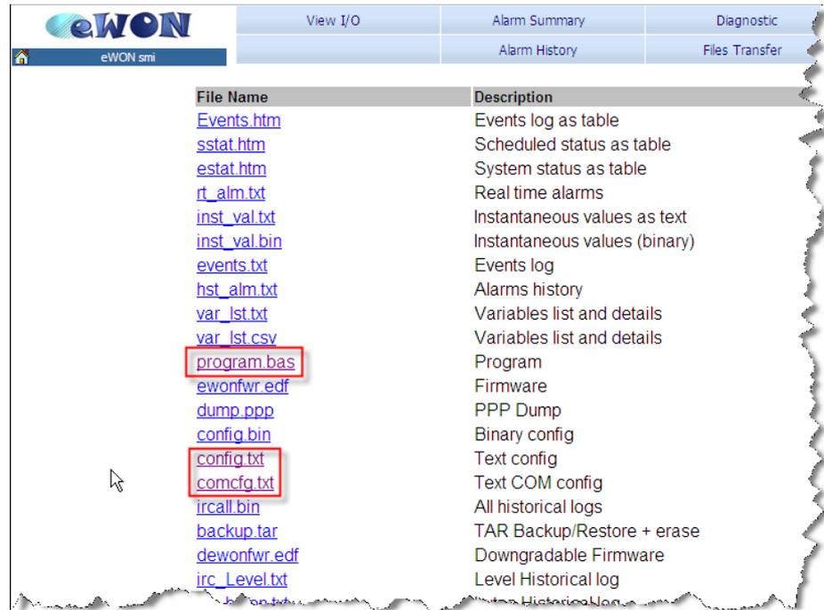
If you click on **config.txt**, the eWON configuration (including the changes that you have made using FTP) will be displayed.
