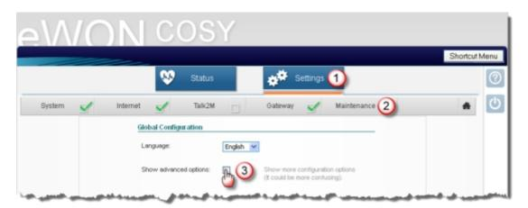
Once checked, the Edit COM Configuration and Edit SYSTEM Configuration links are displayed. The eWON advanced configuration parameters are spread over these tow options. Note: if you do not find a given parameter under one link, check the other.
