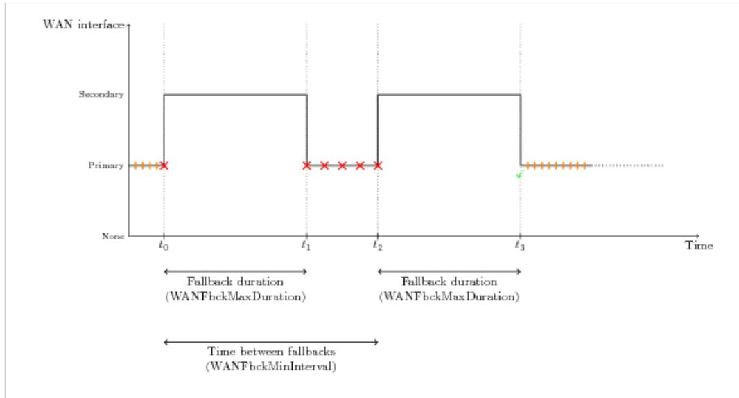
**Fig. 7** Example explained of a WAN fallback
