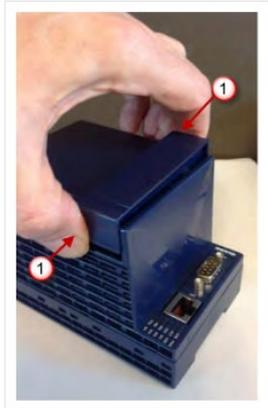
**1** Hooks to be pressed are off-centered. Press while pulling upwards
