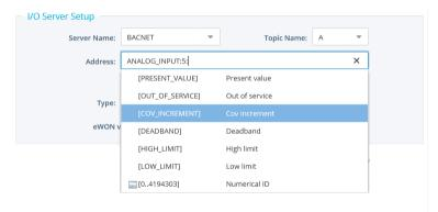
An object is composed of different properties. These properties can be accessed through different Tags.
