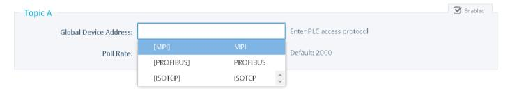
According to the IOserver you selected, Ewon will display the different possibilities for the PLC device address. For example, for some IO servers you first need to specify the protocol that will be used for the polling.
