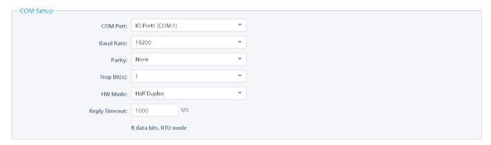
If more than one Serial port is available, you must choose on which COM the MODBUS request will be sent. This example of configuration shows an RS485 setup.
